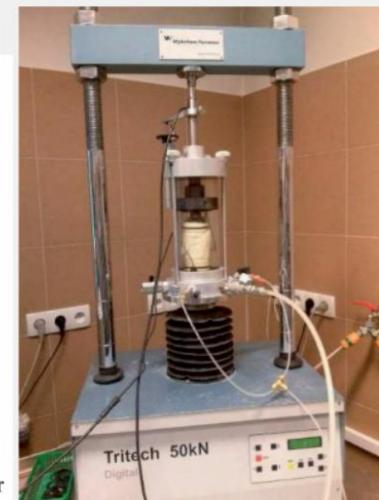
Fig. 7. Designed specifically for the sample dimensions elements supporting the radial strain sensor
